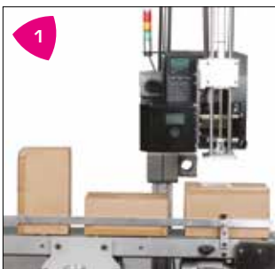
1 Labeling in motion, different sized products up to 30 labels per minute.
